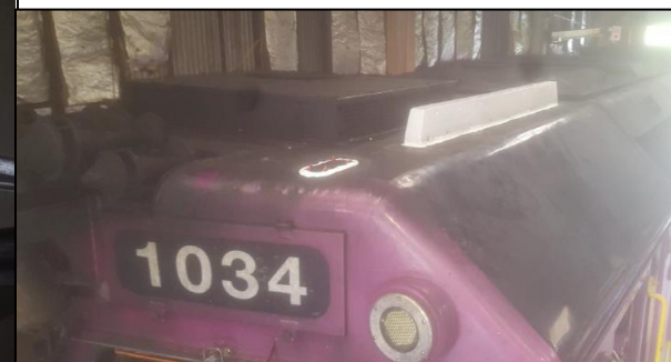
Rooftop Antenna installed
